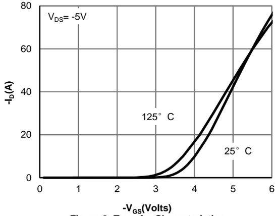
**Figure 2: Transfer Characteristics**
