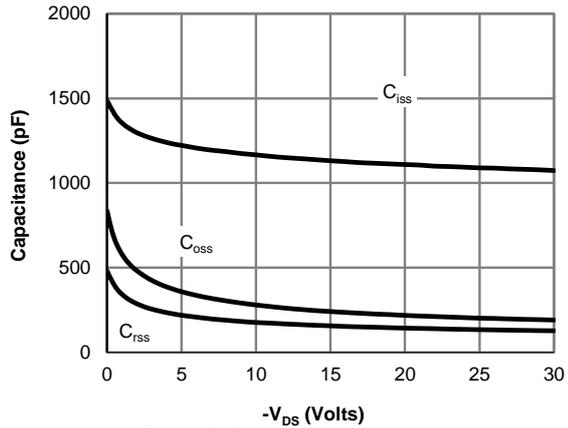
Figure 8: Capacitance Characteristics
