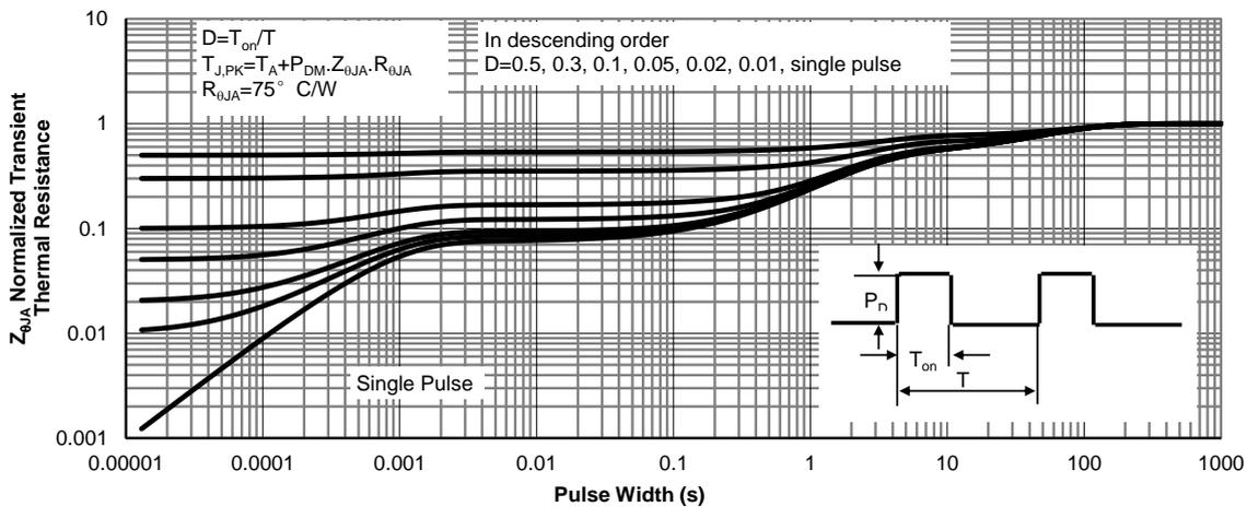
Figure 11: Normalized Maximum Transient Thermal Impedance (Note E)
