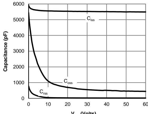
**Figure 8: Capacitance Characteristics**
