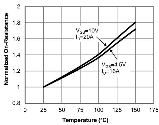
**Figure 4: On-Resistance vs. Junction Temperature (Note E)**
