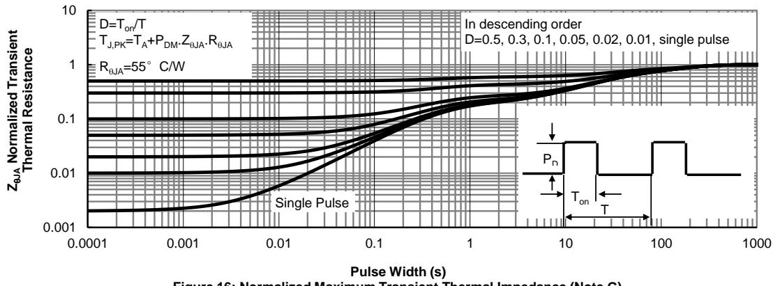
Figure 16: Normalized Maximum Transient Thermal Impedance (Note G)
