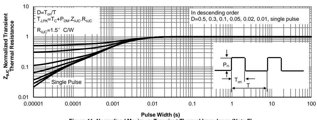
**Figure 11: Normalized Maximum Transient Thermal Impedance (Note F)**
