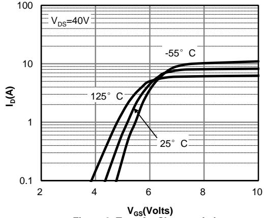
**Figure 2: Transfer Characteristics**
