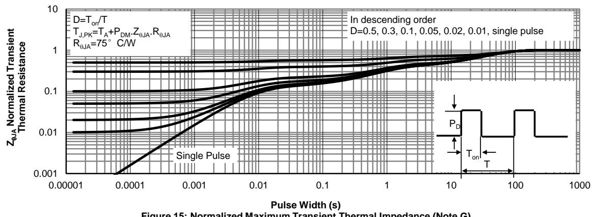
**Figure 15: Normalized Maximum Transient Thermal Impedance (Note G)**
