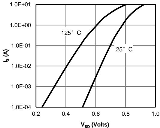
**Figure 6: Body-Diode Characteristics**
