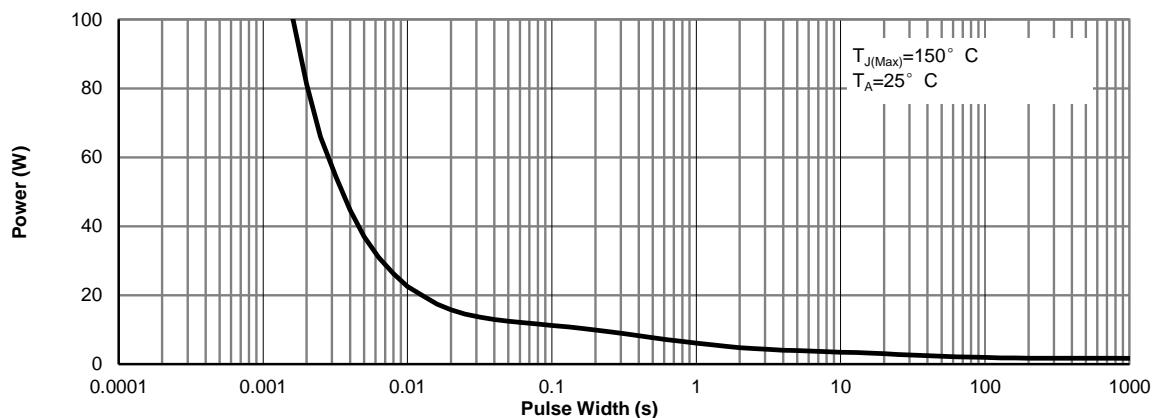
**Figure 14: Single Pulse Power Rating Junction-to-Ambient (Note G)**
