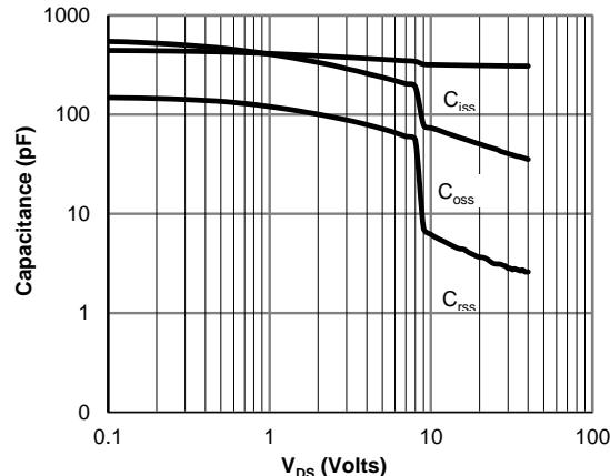
**Figure 8: Capacitance Characteristics**
