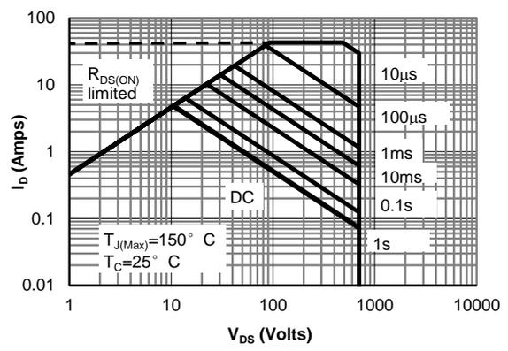
**Figure 10: Maximum Forward Biased Safe Operating Area for AOTF11N70 (Note F)**
