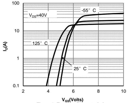
**Figure 2: Transfer Characteristics**
