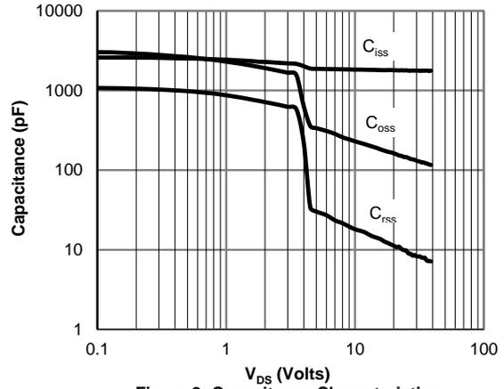
**Figure 8: Capacitance Characteristics**
