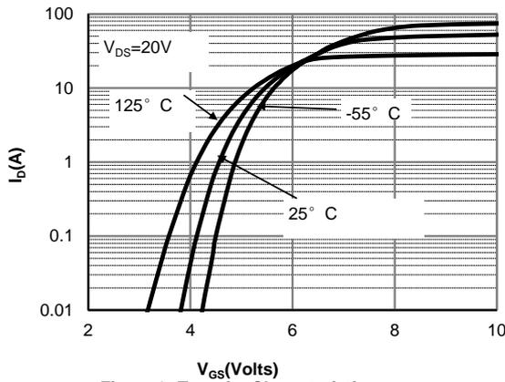
Figure 3: Transfer Characteristics
