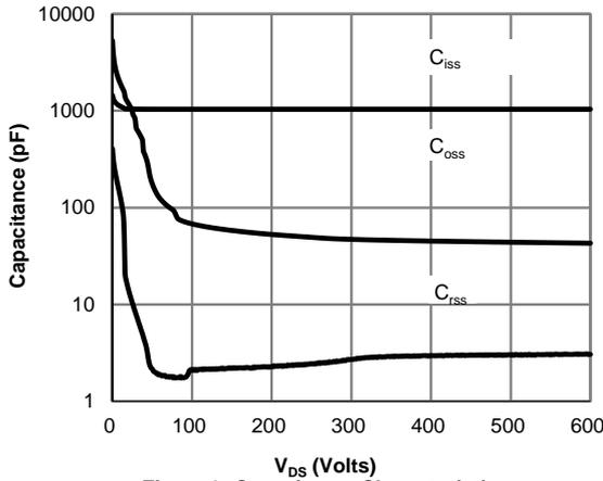
Figure 9: Capacitance Characteristics
