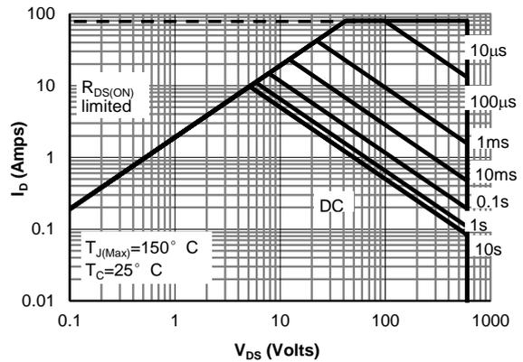
Figure 12: Maximum Forward Biased Safe Operating Area for AOTF20S60L (Note F)
