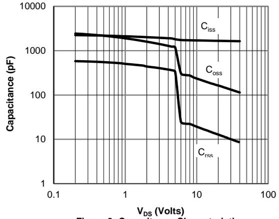
**Figure 8: Capacitance Characteristics**
