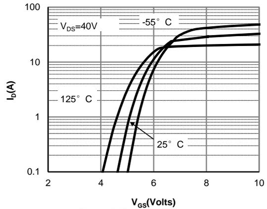
**Figure 2: Transfer Characteristics**
