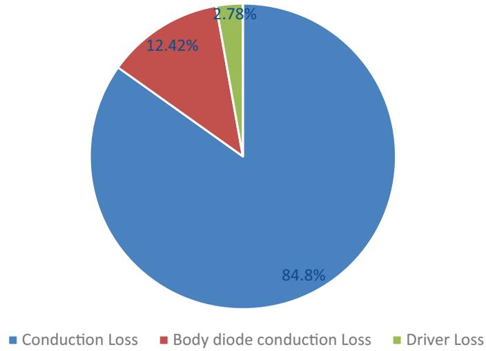
**Figure 12. Power Dissipation of one Phase Low-Side MOSFET**
