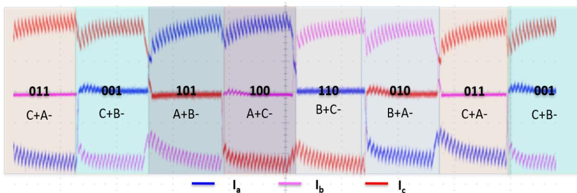
**Figure 2. Commutation Waveforms of a 3-Phase Inverter**
