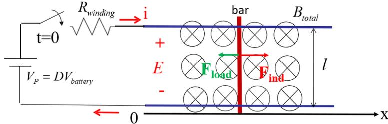
Figure 3. The Simplified Model of a BLDC Motor
