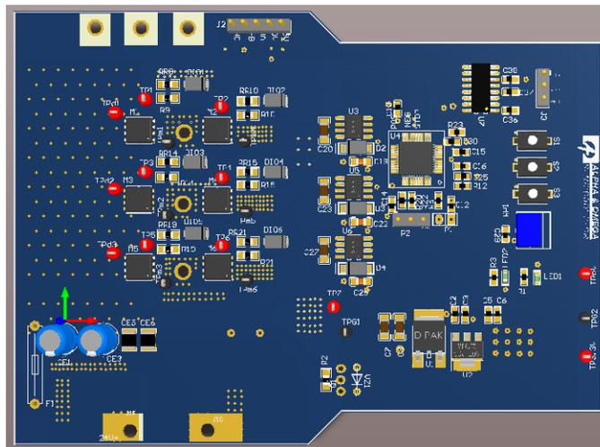
**Figure 9. The BLDC Evaluation Board**
