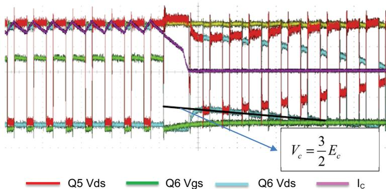
Figure 5. Commutation Wave during Q1 is off, Q2 and Q4 is on
