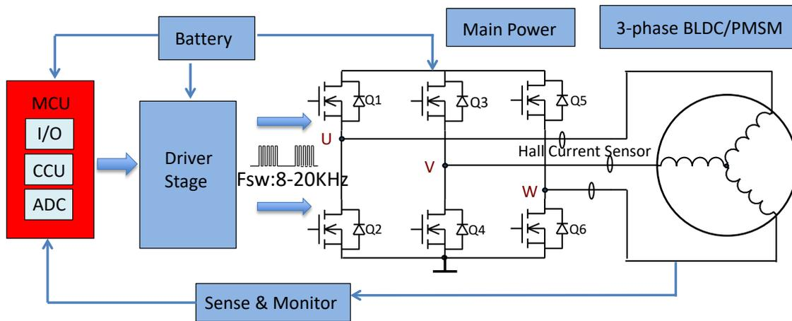
Figure 1. The Block Diagram Brushless DC Motors Control Applying to Power Tool
