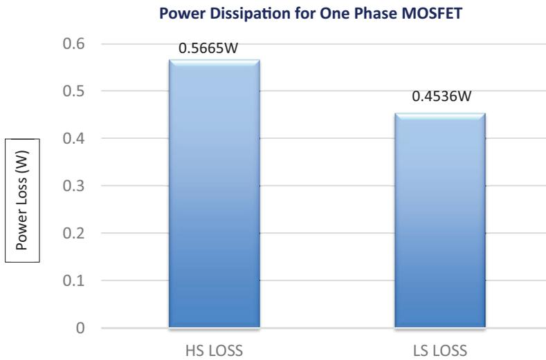
**Figure 13. Total Power Loss of One High and Low Side MOSFET**
