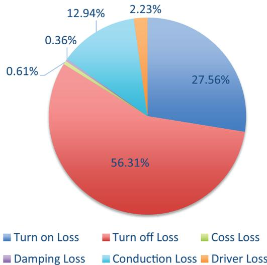
Figure 11. Power Dissipation of one Phase High-Side MOSFET
