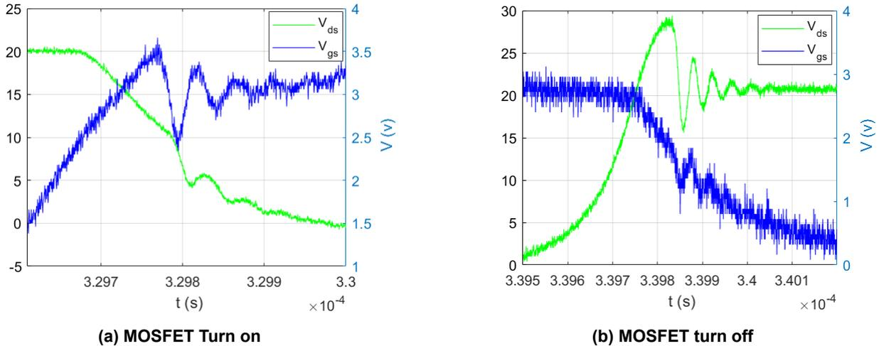
Figure 10. MOSFET AON6500 Turn on and off Waveform
