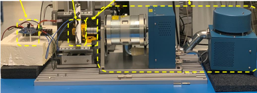
**Figure 8. The BLDC Motor Testing Set-Up**
