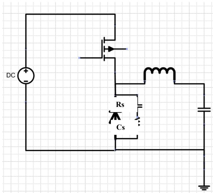
**Figure 1: RC snubber in EZBuck circuit**
