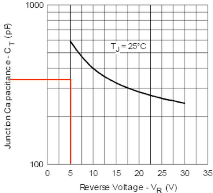
**Figure 5: Junction capacitor of Schottky diode**
