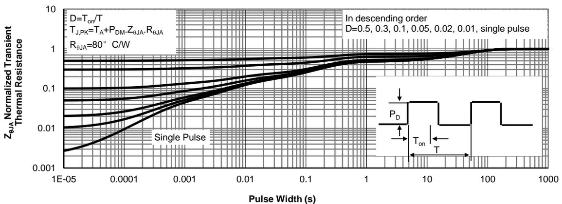
**Figure 11: Normalized Maximum Transient Thermal Impedance (Note H)**
