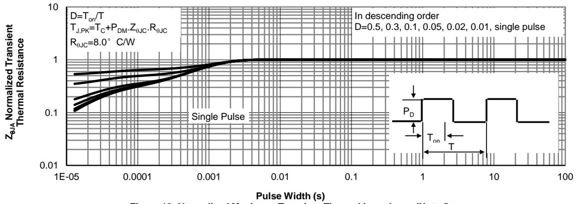
Figure 12: Normalized Maximum Transient Thermal Impedance (Note G)
