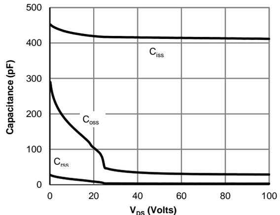
**Figure 8: Capacitance Characteristics**
