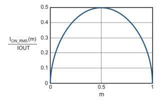
Figure 2. I<sub>CIN</sub> vs. Voltage Conversion Ratio
