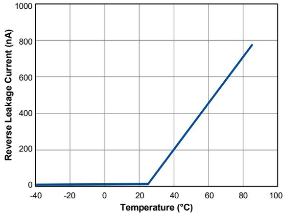
Figure 17. Reverse Leakage Current vs. Temperature
