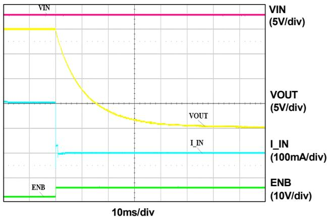
Figure 7. Shutdown (VIN=20V)
