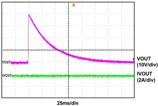
**Figure 13. IEC61000-4-5: 40V Surge Voltage without Device**
