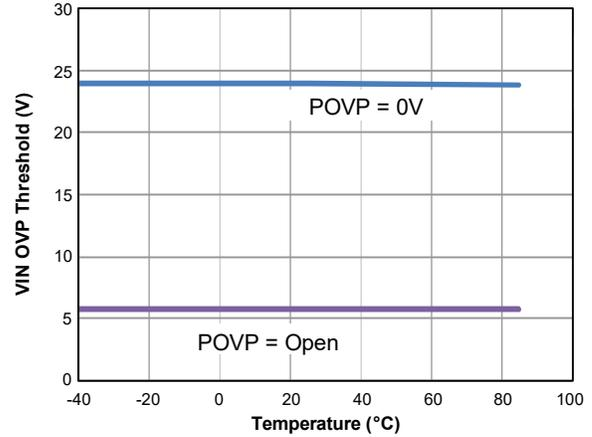
Figure 18. VIN OVP vs. Temperature ( $I_{VOUT}=1\text{A}$ )
