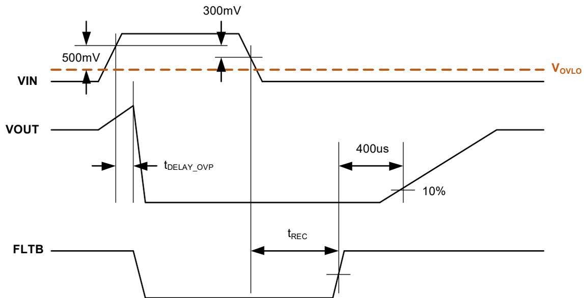
Figure 2. OVP Delay and Recovery Time (AOZ1324DI-01)
