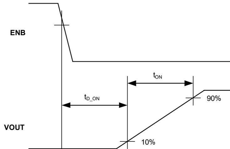
Figure 1. Turn-on Delay and Turn-on Time
