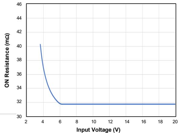
Figure 20. ON Resistance vs. VIN ( $I_{VOUT}=1\text{A}$ )
