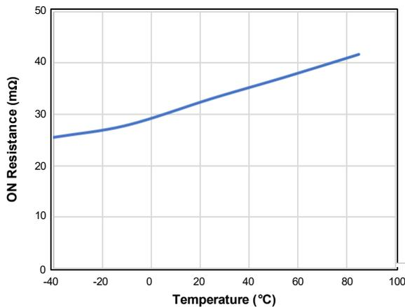
Figure 19. On Resistance vs. Temperature
