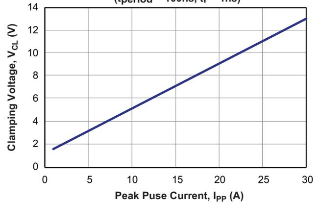
+8kV ESD Clamping Per IEC 61000-4-2
