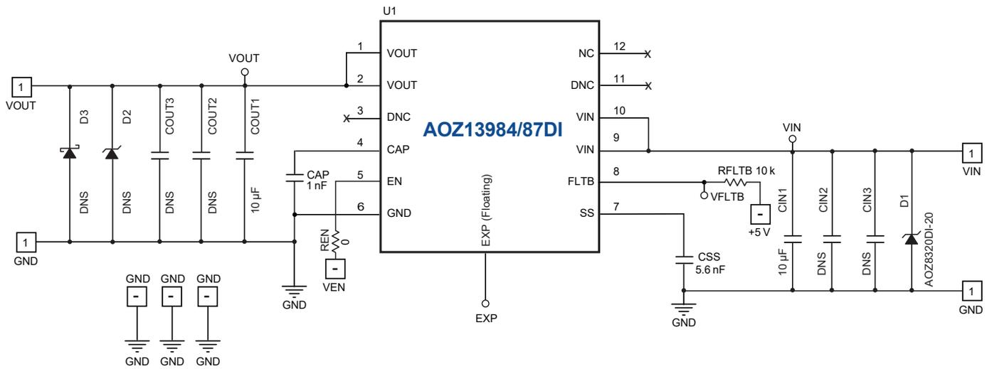
Figure 4. AOZ13984/87DI EVB Schematic
