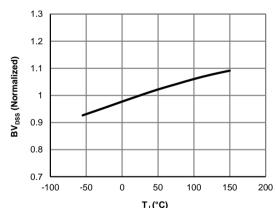
$T_J(^{\circ}C)$  Figure 5: Break Down vs. Junction Temparature
