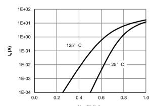
V<sub>SD</sub> (Volts) Figure 6: Body-Diode Characteristics
