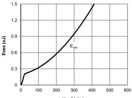
V<sub>DS</sub> (Volts) Figure 9: Coss stored Energy
