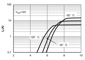
V<sub>GS</sub> (Volts) Figure 2: Transfer Characteristics
