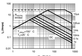
$V_{\rm DS}$  (Volts) Figure 11: Maximum Forward Biased Safe Operating Area (Note F)
