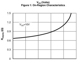
$\label{eq:local_local} I_{D}\left(\mathbf{A}\right)$  Figure 3: On-Resistance vs. Drain Current and Gate Voltage
