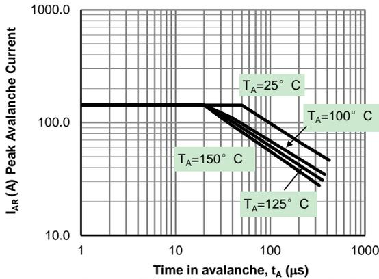
**Figure 9: Single Pulse Avalanche capability (Note C)**
