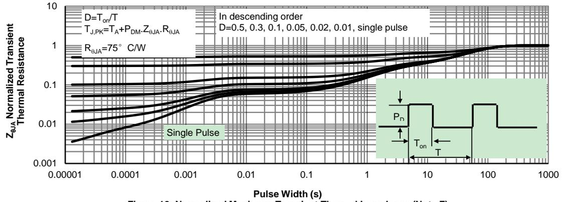
**Figure 12: Normalized Maximum Transient Thermal Impedance (Note F)**
