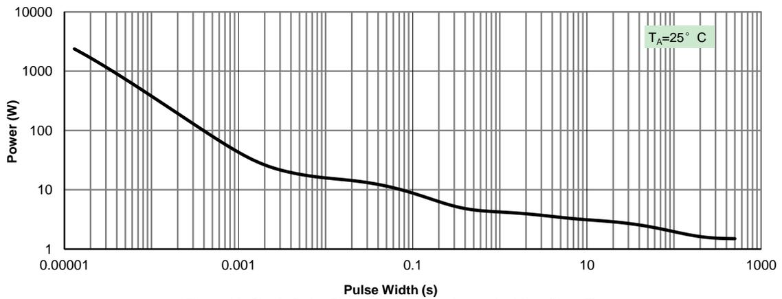
**Figure 11: Single Pulse Power Rating Junction-to-Ambient (Note F)**
