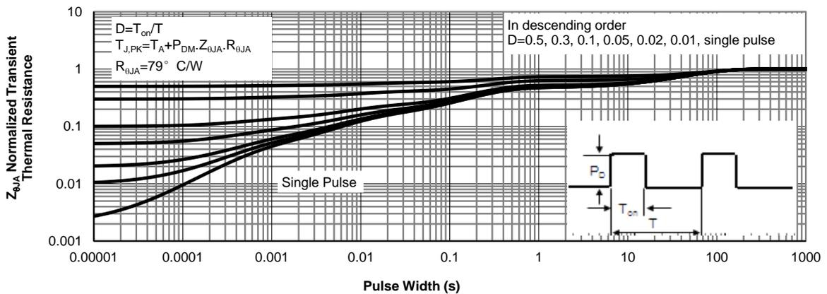
**Figure 11: Normalized Maximum Transient Thermal Impedance (Note H)**
