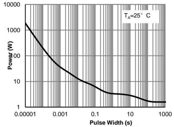
**Figure 10: Single Pulse Power Rating Junction-to-Ambient (Note H)**
