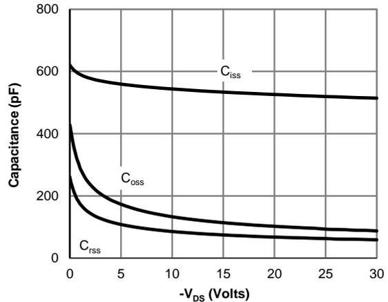
**Figure 8: Capacitance Characteristics**
