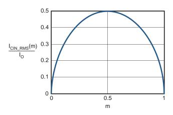
Figure 2. I<sub>CIN</sub> vs. Voltage Conversion Ratio
