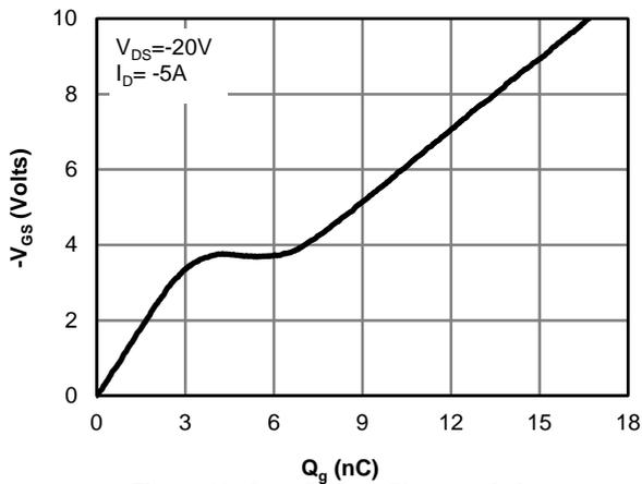
Figure 18: Gate-Charge Characteristics
