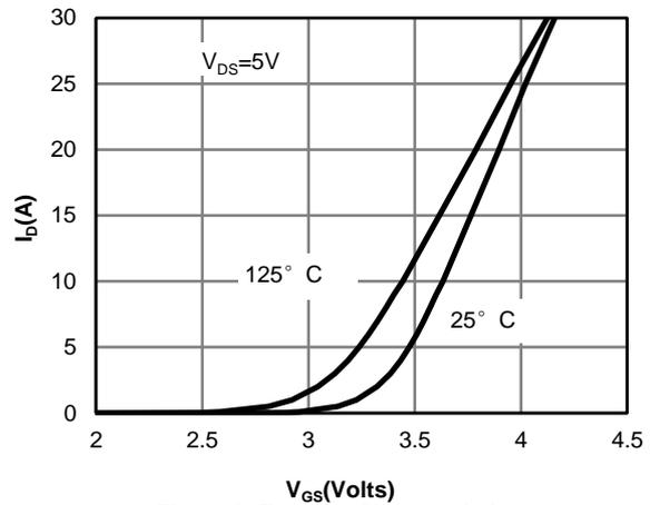
**Figure 2: Transfer Characteristics**
