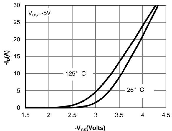
**Figure 13: Transfer Characteristics**
