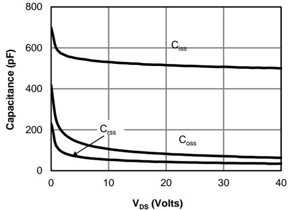
**Figure 8: Capacitance Characteristics**
