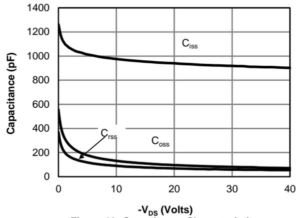
Figure 19: Capacitance Characteristics
