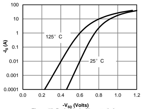
**Figure 17: Body-Diode Characteristics**
