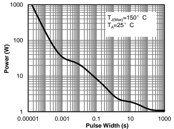
Figure 21: Single Pulse Power Rating Junction-to-Ambient (Note E)
