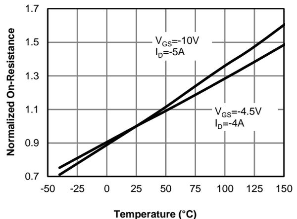
**Figure 15: On-Resistance vs. Junction Temperature**
