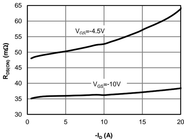
**Figure 14: On-Resistance vs. Drain Current and Gate Voltage**
