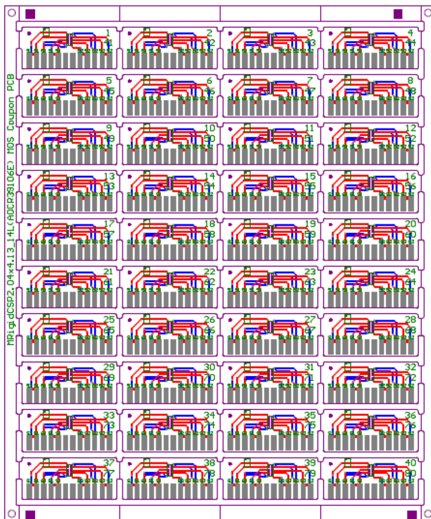
Figure 44. Example of Coupon PCB Board for on-board Warpage Measurement
