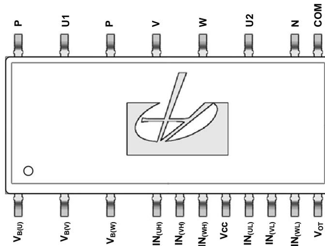
**Figure 1. Pin Configuration**
