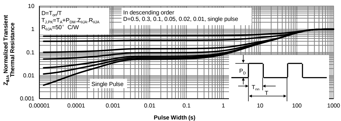
Figure 16: Normalized Maximum Transient Thermal Impedance (Note H)
