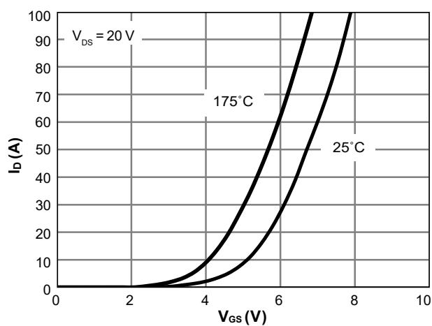
Figure 5. Transfer Characteristics
