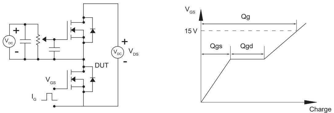
Figure 18. Gate Charge Test Circuits and Waveforms
