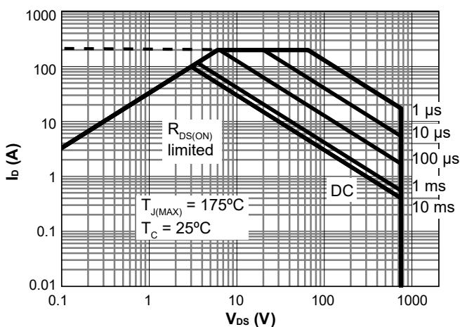
Figure 16. Maximum Forward Biased Safe Operating
