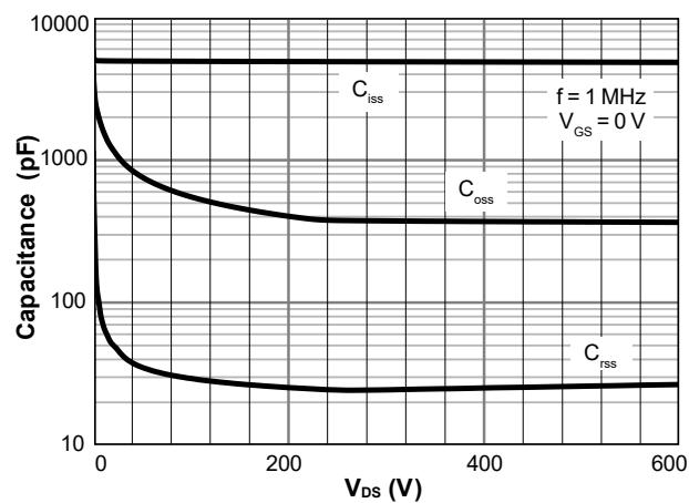
Figure 10. Capacitance Characteristics
