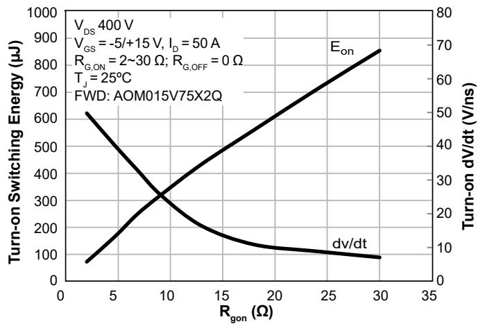
Figure 13. Turn-On Energy and  $dV/dt$  vs.
