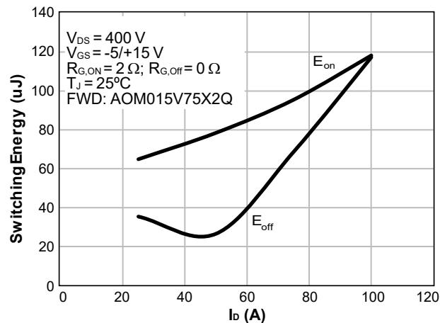
Figure 12. Switching Energy vs. Drain Current
