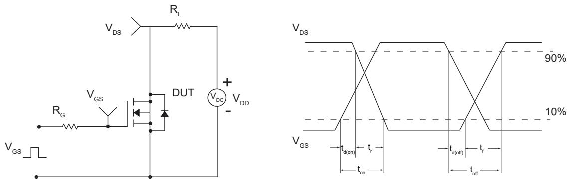
Figure 19. Resistive Switching Test Circuit and Waveforms
