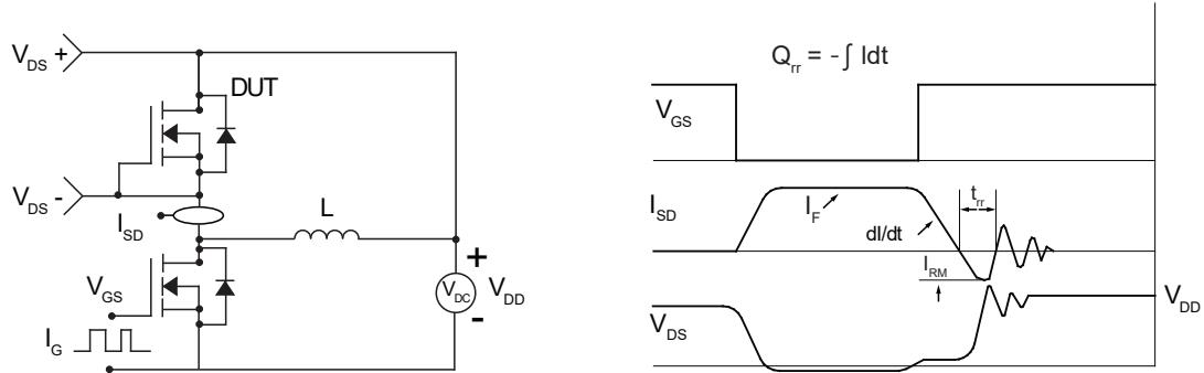
Figure 21. Diode Recovery Test Circuits and Waveforms
