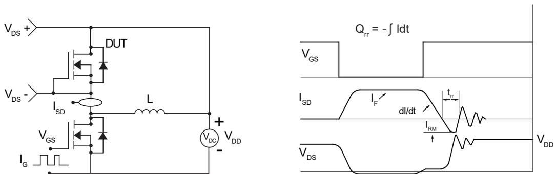
Figure 22. Diode Recovery Test Circuits and Waveforms
