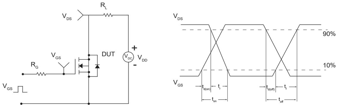
Figure 20. Resistive Switching Test Circuit and Waveforms
