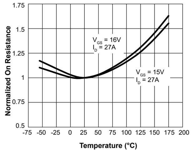
Figure 4. Normalized On Resistance vs. Junction Temperature
