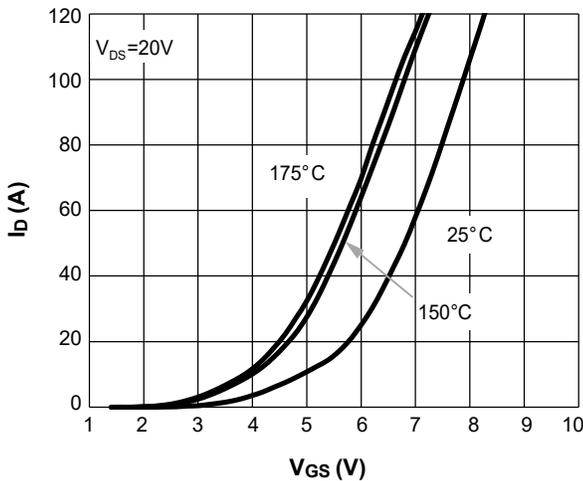
Figure 5. Transfer Characteristics
