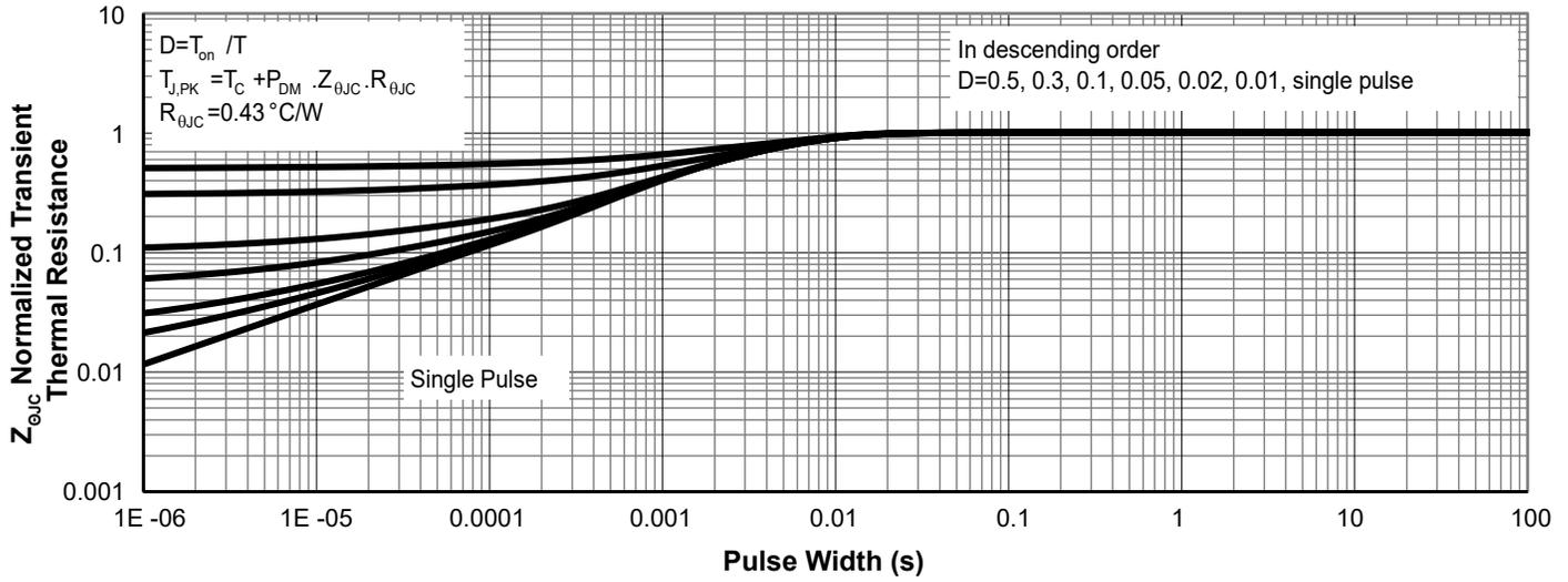
Figure 18. Normalized Maximum Transient Thermal Impedance for AOM020V120X2 (Note I)
