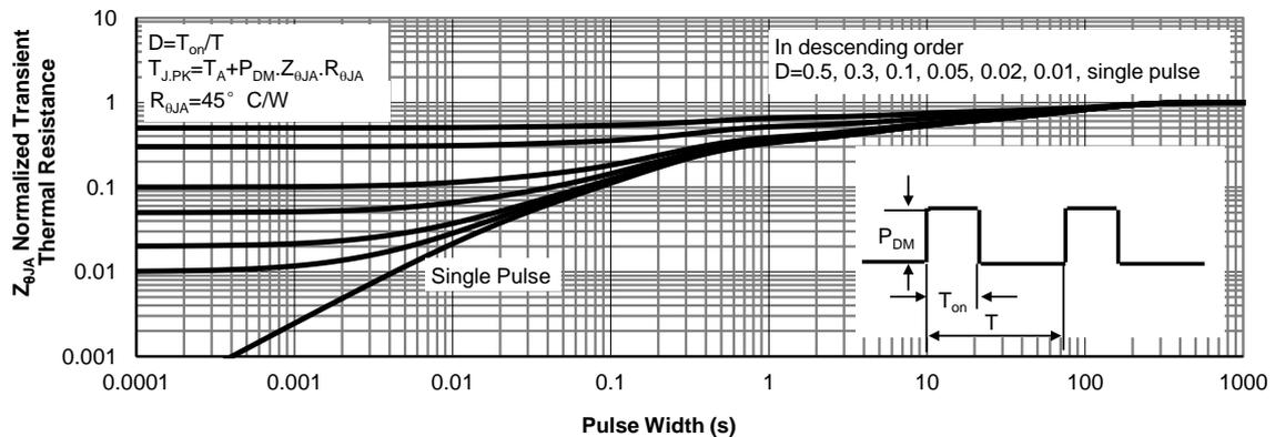
Figure 15: Normalized Maximum Transient Thermal Impedance (Note G)
