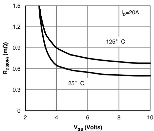
**Figure 5: On-Resistance vs. Gate-Source Voltage (Note E)**
