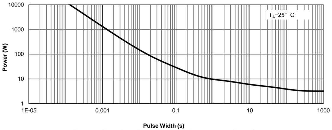
Figure 14: Single Pulse Power Rating Junction-to-Ambient (Note G)
