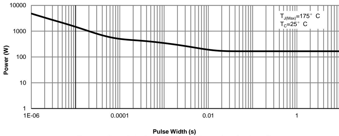
**Figure 16: Single Pulse Power Rating Junction-to-Case-Top (Note F)**
