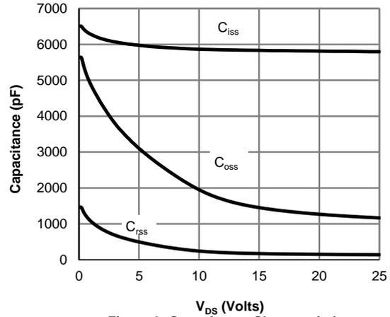
**Figure 8: Capacitance Characteristics**
