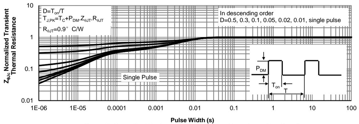
**Figure 17: Normalized Maximum Transient Thermal Impedance-Top (Note F)**
