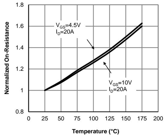
**Figure 4: On-Resistance vs. Junction Temperature (Note E)**
