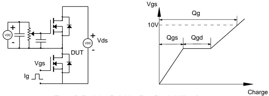
Figure B: Resistive Switching Test Circuit & Waveforms
