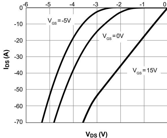
Figure 8. Body-diode Characteristics  $T_J = 175^\circ\text{C}$
