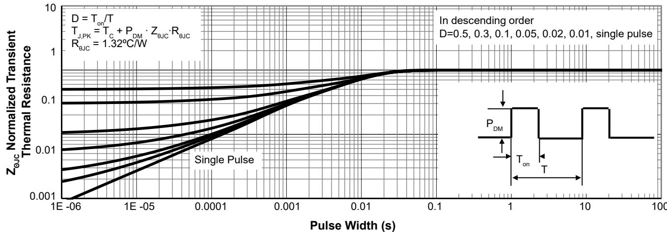
Figure 17. Normalized Maximum Transient Thermal Impedance for AOTL040V65X2 (Note I)
