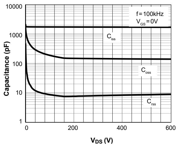
Figure 10. Capacitance Characteristics
