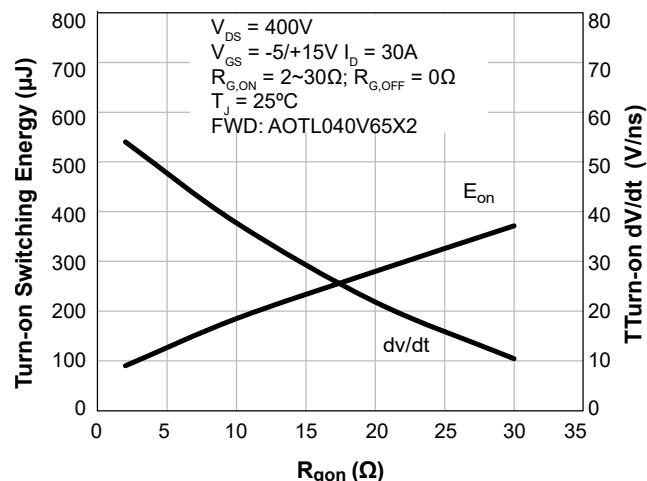
Figure 13. Turn-On Energy and  $dV/dt$  vs.
