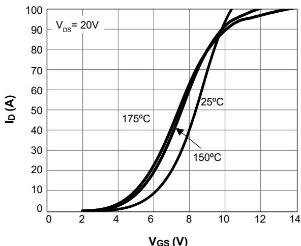
Figure 5. Transfer Characteristics
