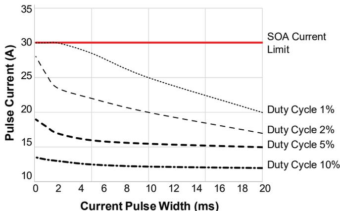
**Figure 11. AOZ13289DI-01 Sinking Switch Pulsed Current vs. Duration for a Given Duty Cycle**
