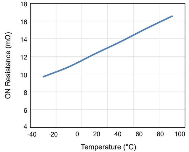
Figure 6. On Resistance vs. Temperature (VIN = 20 V)
