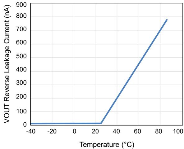
Figure 7. V<sub>OUT</sub> Reverse Current Leakage vs. Temperature
