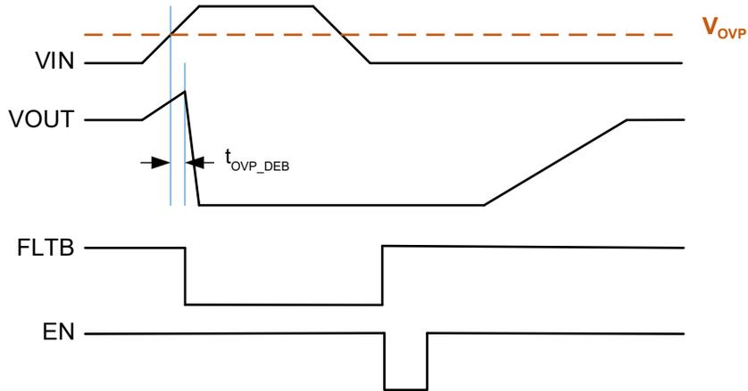
Figure 2. Over-Voltage Protection
