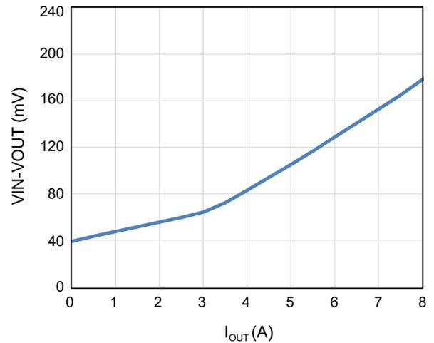
Figure 8. Ideal Diode Regulation Voltage vs. I<sub>OUT</sub>
