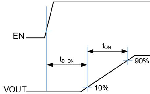
Figure 1. Turn-on Delay and Turn-on Time
