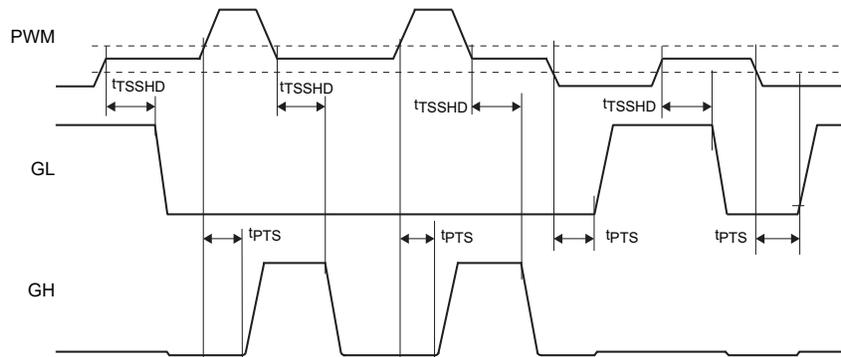
Figure 2. PWM Tri-State Input Logic Timing Diagram
