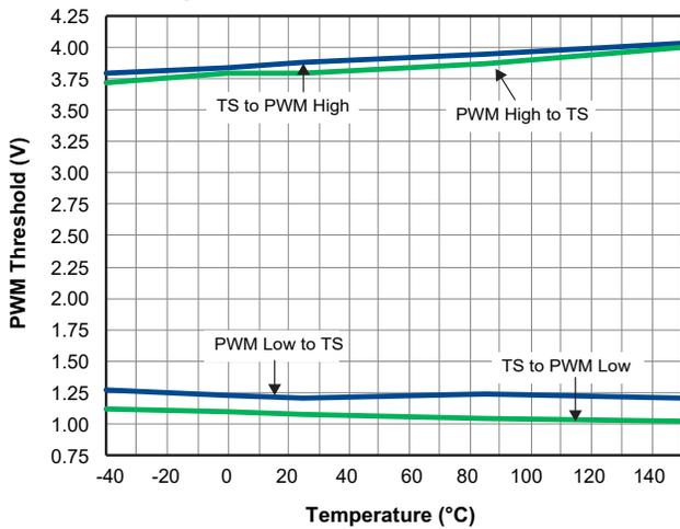
Figure 7. FCCM Input Threshold vs. Temperature
