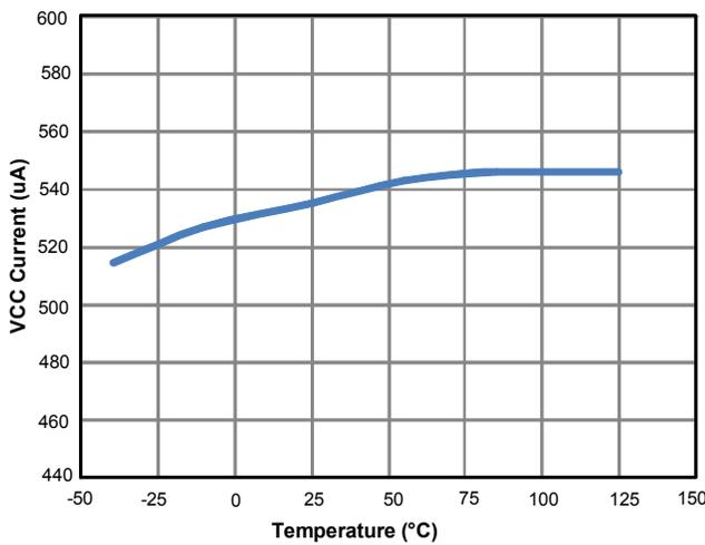
Figure 5. Supply Current ( $I_{VCC}$ ) vs. Temperature
