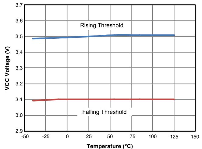
Figure 8. UVLO ( $V_{CC}$ ) Threshold vs. Temperature
