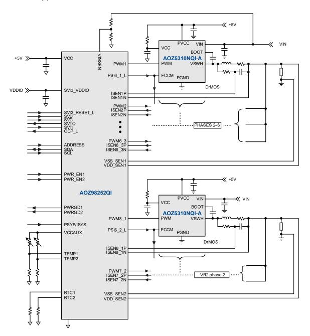
Figure 1. AOZ98252QI Typical Application Diagram
